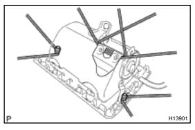
(2) Wind the wire harness around the bolts, and pass the wire harness though the installation holes.
