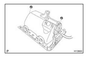
(1) Install the front passenger airbag assembly with the 2 nuts.
