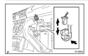
(c) Disconnect the airbag connector.
