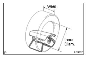
side the tire with the airbag deployment side facing inside.
